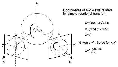
Fig. 1. Determination of coronal loop height via triangulation. Coronal loop as seen from two view points separated in the ecliptic by stereo angle  $\alpha$ . The coordinates in the plane of the sky for the two views are related by a simple rotational transform and the complete 3D geometry of the loop can be determined from the measured (x,y) and (x',y') as shown.
