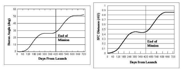
**Fig. 3: Left: Stereo (Earth-Sun-S/C) Angle vs. Flight Time** shows S/C dwells near 25° stereo angle. Right: Spacecraft distance from Earth vs. flight time.
