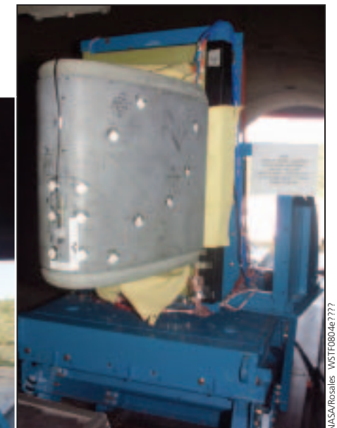
Hypervelocity Impact Testing of RCC Wing Leading Edge.
