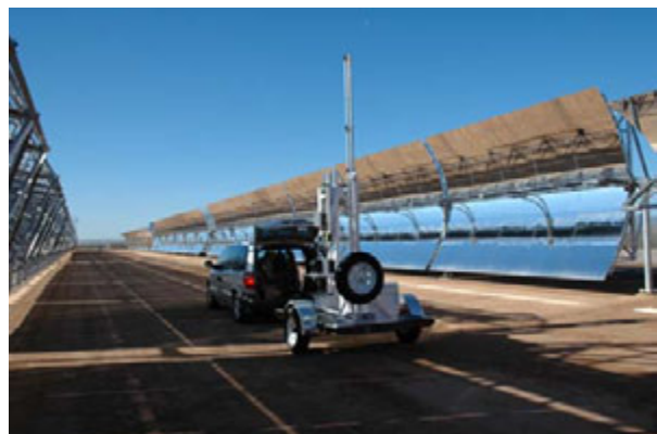
Fig. 6. Prototype TOP alignment system under test at the APS Saguaro parabolic trough plant.
