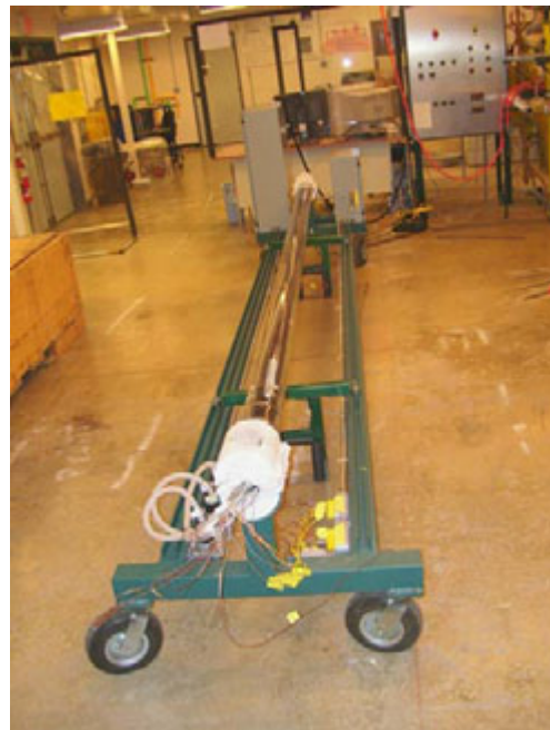
Fig. 8. New parabolic trough receiver thermal loss test bed
