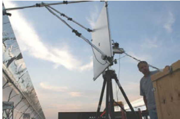
Fig. 10. Optical testing of LS-3 concentrator at SEGS IX with VSHOT
