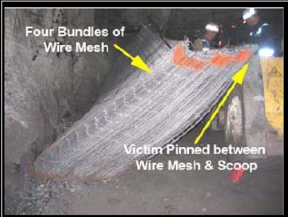
On Saturday, January 6, 2007, at approximately 12:30 p.m. a 26 year old utilityman, was fatally injured when welded wire mesh panels (also referred to as screens) fell over, pinning him against a diesel-powered scoop. The miner was attempting to remove one of the four bundles of wire mesh panels by cutting the steel banding
