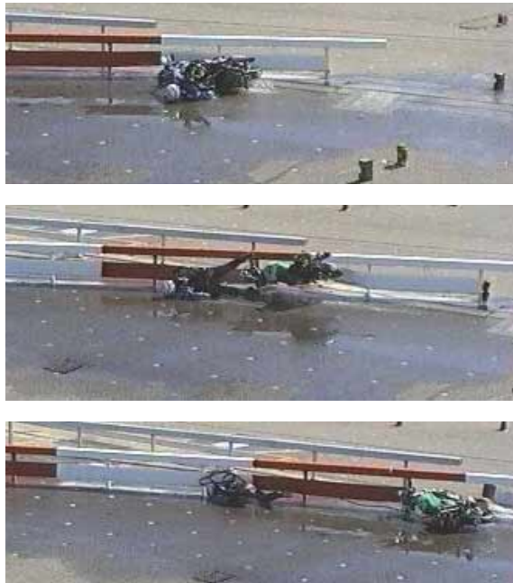
Figure 17. Full-scale crash test where the sliding motorcycle impacted the modified steel guard rail system
