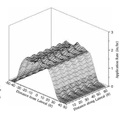
Composite application rate pattern under a center pivot from rotating-type sprinklers on an offset boom having a 15-foot horizontal projection on both sides of the center pivot lateral with 10-foot sprinkler spacing and 10
