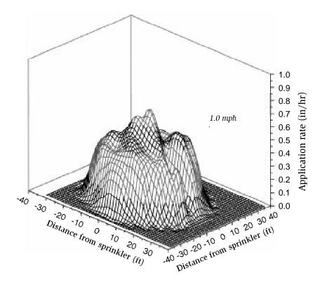
The application rate pattern from a wobbling-plate type sprinkler having 9 grooves and a 15–degree trajectory angle is shown in figure 7. This application rate pattern resembles a truncated cone with an additional elliptical shaped peak near the sprinkler. The application rate pattern is very uniform except near the sprinkler.
