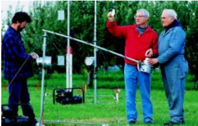
Electronic technician Barry Nudd (left) and agricultural engineers Ross Brazee (right) and Robert Fox inspect a collection filter from a high-volume air sampler.
