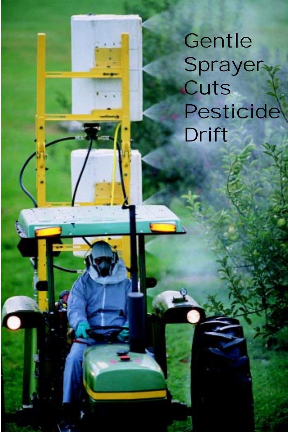
The air-curtain orchard sprayer driven by technician Andrew Doklovic uses multiple crossflow fans to disperse pesticide to apple trees. Under some conditions, the smoother, gentler flow of air can reduce spray drift by half.
