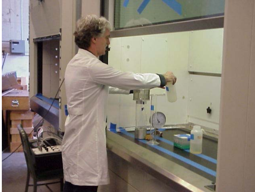
Fig. 8 – HAM Test Series – Conventional hood – Left ejector; exchanging objects.
