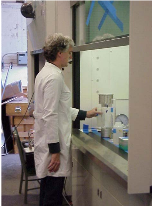
Fig. 9 – HAM Test Series – Conventional hood – Left ejector; replacing object after rotating.
