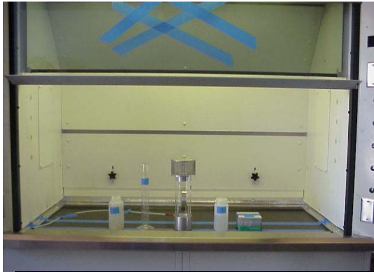
Fig. 1 – HAM Test Series – Conventional hood – Center ejector; object’s starting position.
