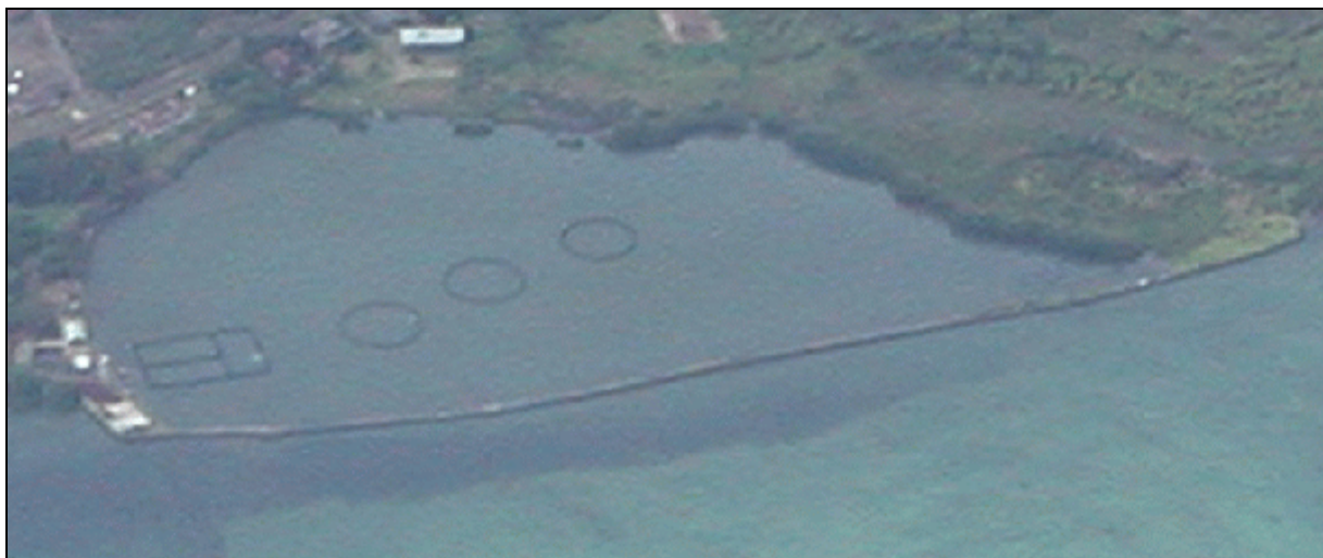
Fig. 65. 'Ualapu'e Fishpond. Note 3 Rectangle 5,000sq Ft. Nursery Net Pens and 3 Round 7,500sq. Ft Grow Out Pens.
