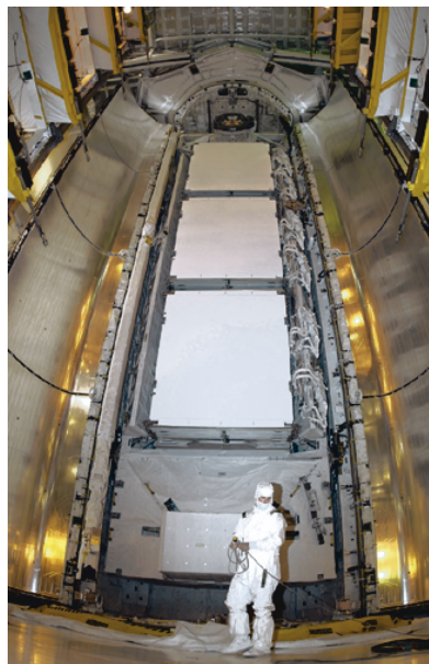
The S1 Truss segment inside Atlantis' payload bay
