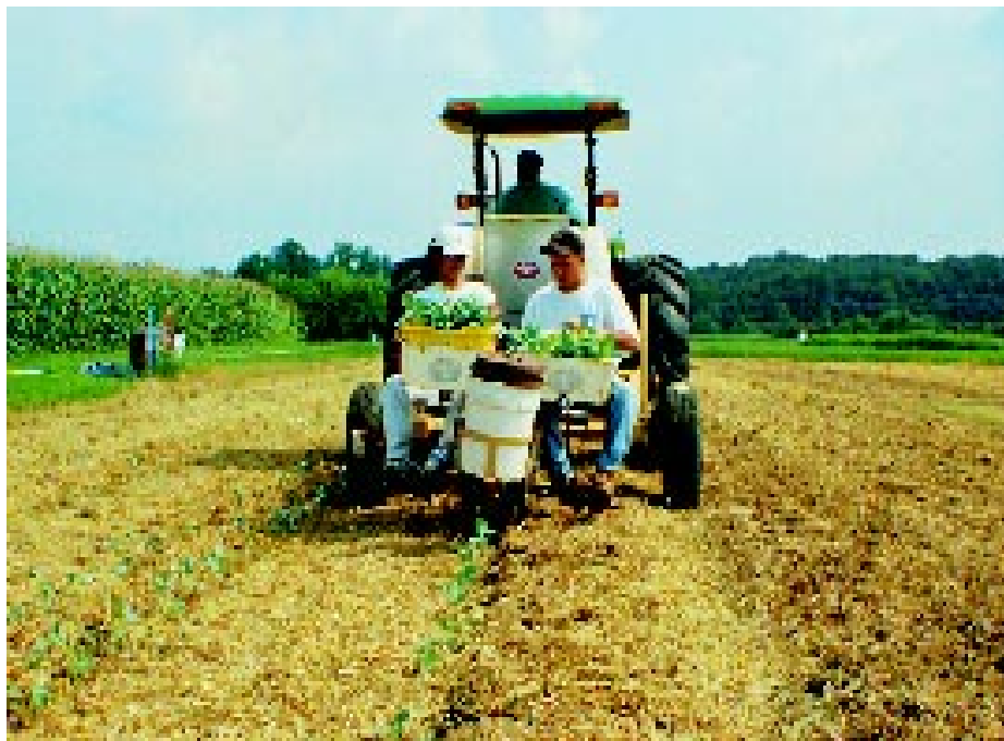
Facing page: The no-till planter that technicians Maria Ballesteros (left) and Christopher Wong are operating cuts through soybean mulch on the surface, opens a furrow in the soil, applies liquid fertilizer, drops the transplant, and then closes the furrow.
