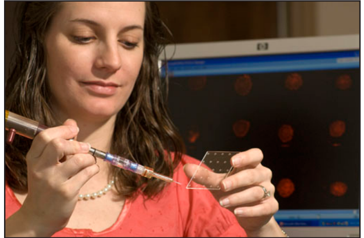
LOCAD scientist Heather Morris loads a sample onto a demonstration microfluidic chip.
