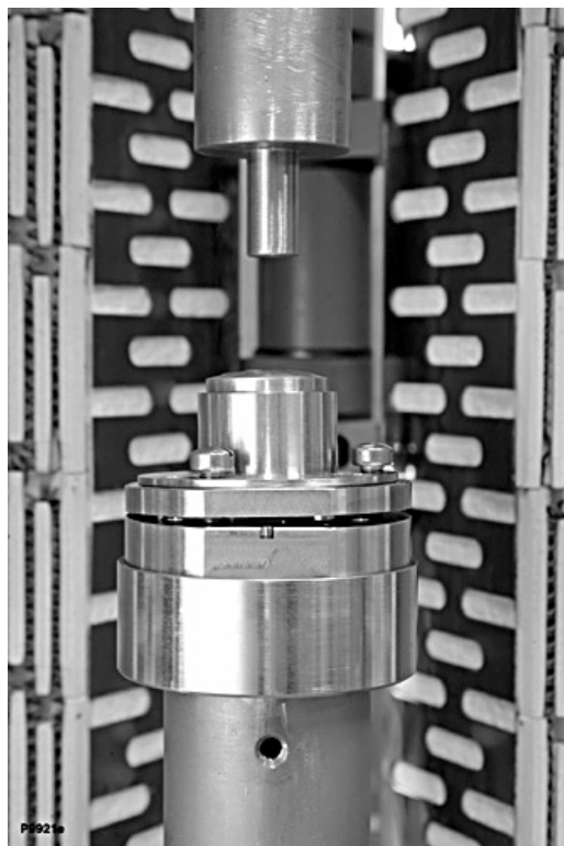
Figure 12. Close up of shear punch fixture and testing platform.
