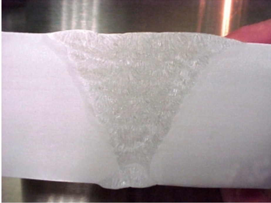
Fig. 1. Macro photograph showing a cross-section view of the submerged arc weldment used for testing and analysis. The P91 plate was 2 in thick.
