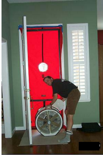
Using a blower door to perform a pressurization test on a building envelope
