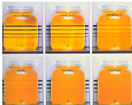
Figure 5: Example of Distillate Fuel Haze Rating Standard Using ASTM Clear and Bright Test
