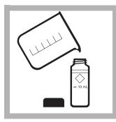
**5.** Fill a second sample cell with 10 mL of sample (the blank).
