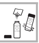
**3.** Add the contents of one SulfaVer 4 Reagent Powder Pillow to the sample cell (the prepared sample). Swirl to mix.
