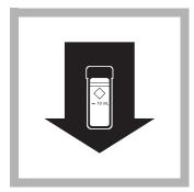
**8.** Within five minutes after the timer beeps, place the prepared sample into the cell holder.
