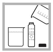
**2.** Fill a sample cell with 25 mL of sample. Collect at least 40 mL of sample in a 50-mL beaker.
