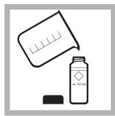
**2.** Fill a clean, round sample cell with 10 mL of sample.
