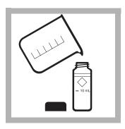
**5.** Fill another sample cell (the blank) with 10 mL of sample.
