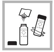
**3.** Add the contents of one FerroVer Iron Reagent Powder Pillow to the sample cell (the prepared sample). Swirl to mix.
