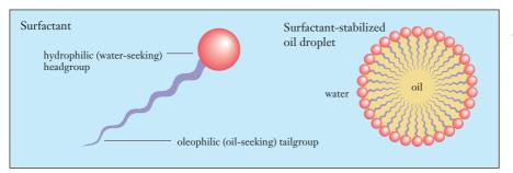
Surfactants consist of two parts; a water-seeking hydrophilic headgroup and an oil-seeking oleophilic tailgroup. This allows them to stabilize oil droplets.
