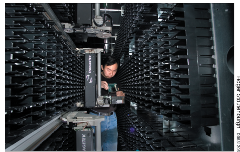
David Yu of the Physics Department inspects the newly acquired 2.4-petabyte robotic tape storage system that will provide increased storage capacity for RHIC and ATLAS computing activities in 2006.
