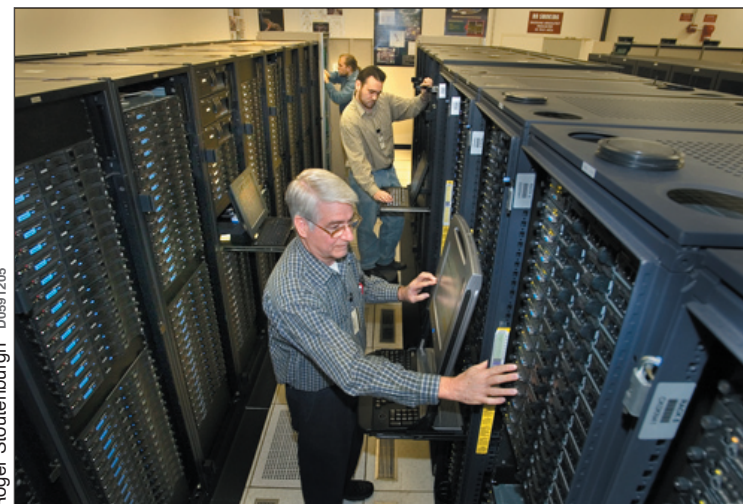
(From front) Richard Hogue, Chris Hollowell, and Alex Withers of the Physics Department service the RHIC/ATLAS Linux Farm of 4000+ processors that provide the bulk of the computational and storage resources for RHIC experiments as well as for U.S. participants in the future ATLAS experiment at CERN.
