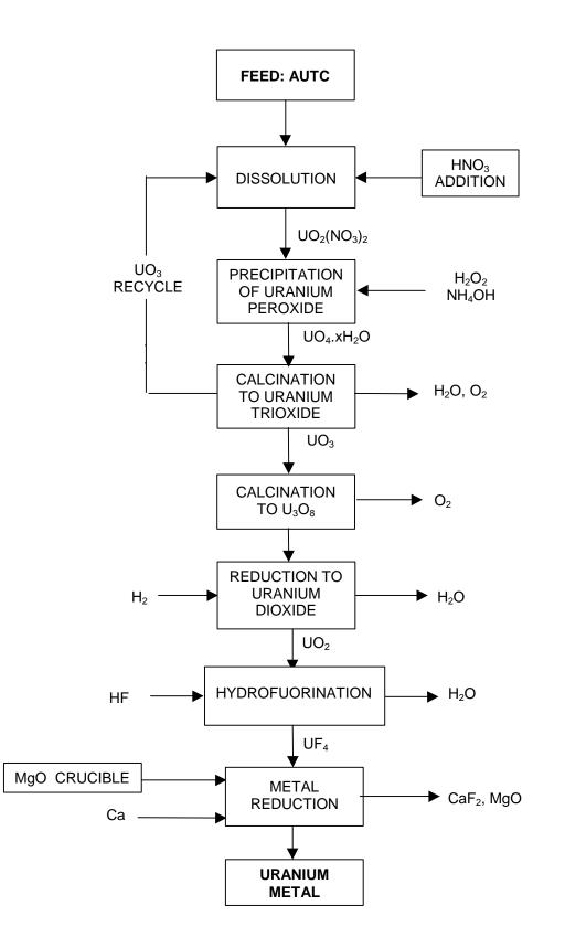
Figure 2. LUE Laboratory. Flow Diagram For Uranium Metal Production.
