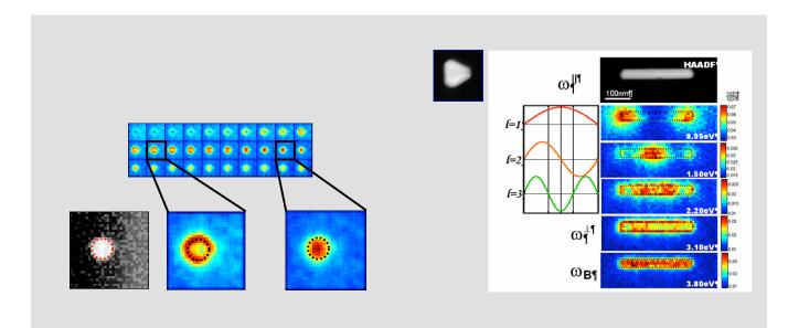
**Figure.** Energy filtered images revealing the signatures of shape dependant plasmonic excitation modes for different silver particles. Spherical particle (left) triangular prism (center) and silver nanorod. (right).
