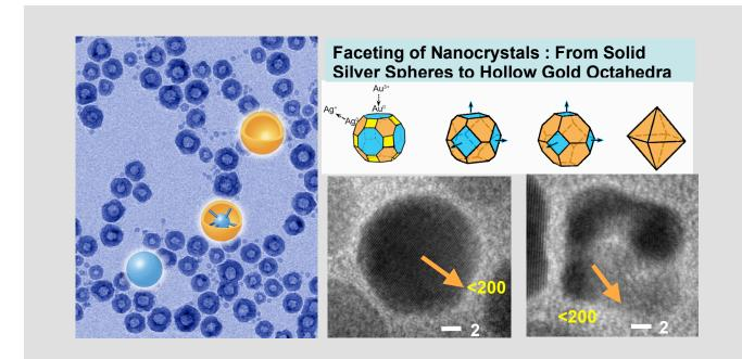
**Figure.** (left) Hollow Cobalt Sulfide Nanocrystals. (right) Transformation of spherical Ad nanocrystals into octahedral hollow Au nanoparticles via galvanic displacement reaction.
