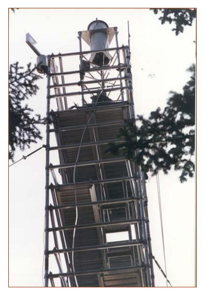
The Automated Cloud Collector (in the down position) on top of the CASTNET tower at Clingmans Dome, TN
