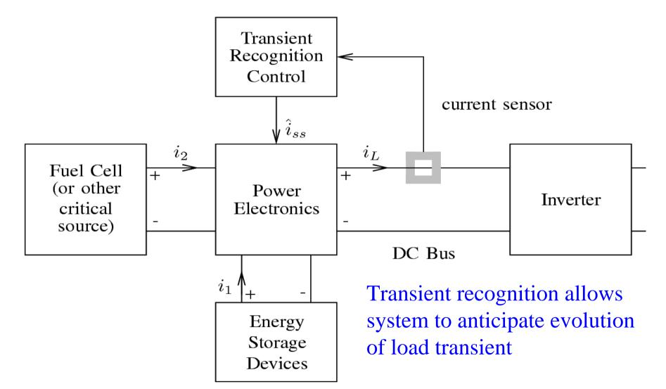
*Transient Recognition Control for Hybrid Fuel Cell Systems,* IEEE Transactions on Energy Conversion
