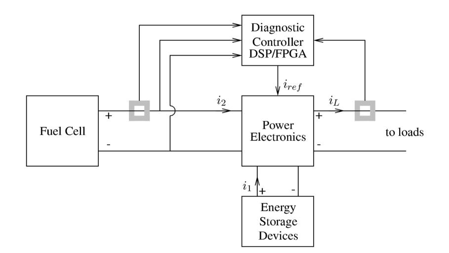
Continuously diagnose fuel cell and adapt control response
