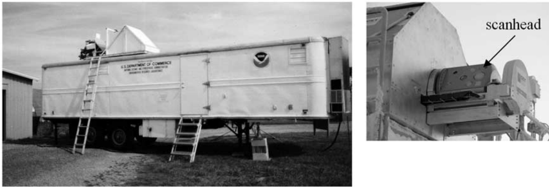
Figure 1. Comparison of a scanning microwave radiometer made more than 25 years ago (left [Snider et al. , 1980; Hogg et al. , 1983]), used by Warner et al. [1986] in a cloud tomography demonstration, with a recently developed Ground-based Scanning Radiometer (right, [Cimini et al. , 2007]) deployed in Barrow, Alaska, USA during 2004. The Snider radiometer operates at two frequencies (23.8 and 31.4 GHz). The scanning bearings are on the top of the trailer; the electronics and antenna are located in the trailer to keep a benign working environment. Ground-based Scanning Radiometer (GSR) is a multi-frequency scanning radiometer operating from 50 to 380 GHz; it can provide unprecedented information on the evolution of temperature, water vapor, and clouds. The photo shows that the scanhead moved out of the framework for atmospheric viewing. The circles are the radiometers of different wavelengths mounted on the scanhead.
