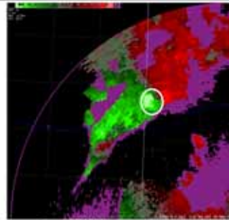
Most likely area for XDW is on up-shear flank of low-level mesocyclone and in the precip-filled RFD area
