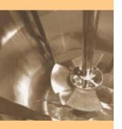
Inside one of four 9000-liter fermentation tanks at the National Renewable Energy Laboratory's Bioethanol Pilot Plant. The facility enables NREL and its industry partners to move advances in producing ethanol and other fuels and chemicals from biomass into the development phase.
