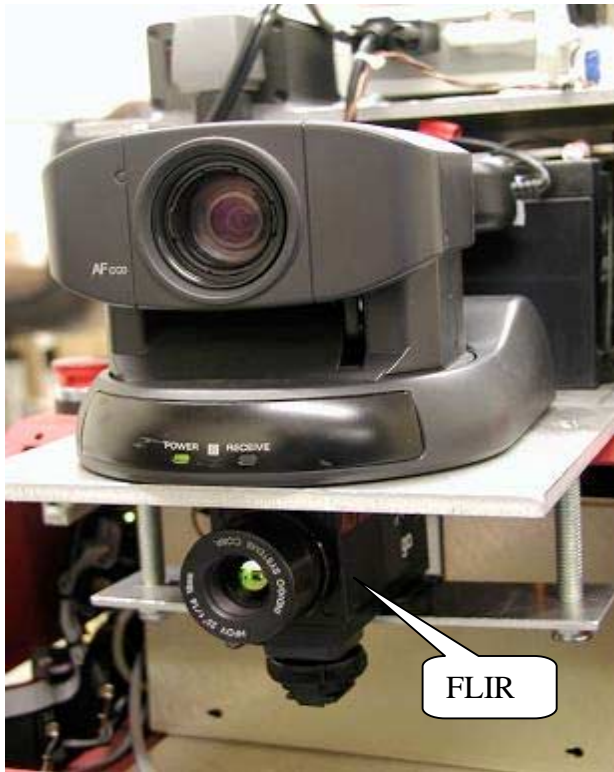
Figure 1: Thermal camera mounted on robot
