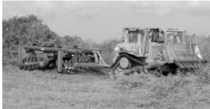
Under control. This roller chopper, pulled by the Service's Natalie Niederost, helps control prescribed burns. FWS photo: Doug Broce.
