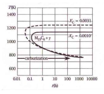
By carburizing below the C-curve for the precipitation of M<sub>23</sub>C<sub>6</sub> colossal carbon supersaturations can be attained.
