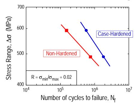
The A286 alloy was initially solutionized for 1 hour at 982°C, oil quenched, then aged 16 hours at 718°C producing a tensile strength of 1100 MPa.
