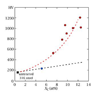
Note at greater than 6 at. pct. (1.3 wt. pct.) the hardness of 316 Stainless Steel increases at a rapid rate with increasing carbon content.
