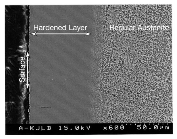
LTCSS treated 316 Stainless Steel etched with Marble's reagent: 10 g CuSO<sub>4</sub>, 50 ml HCl, and 50 ml H<sub>2</sub>O.
