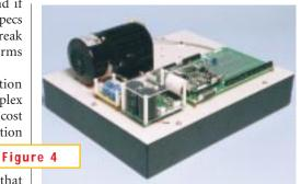
For advanced motor-control-algorithm development, use the real thing: The Motionpro DSP AC331 development system from Applied Microelectronics takes you from ac mains, through DSP, to a <sup>1</sup>/<sub>5</sub>-hp single-phase induction motor.
