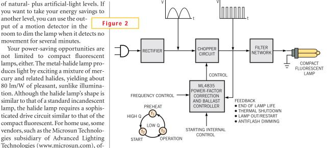
The compact-fluorescent-lamp controller must provide different functions in the three key cycles of the lamp's operation; it can also provide advanced end-of-life, thermal-shutdown, and dimming functions, all matched to the bulb type.
