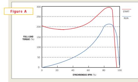
The torque-versus-speed curve for a typcial single-phase induction motor shows the rapid falloff in torque outside the 80 to 90% synchronous-speed band (adapted from Reference A).
