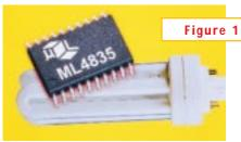
Using the Micro Linear ML4835 as a controller, you can build an efficient and versatile electronic ballast for compact fluorescent lamps, which can replace incandescent lamps in many consumer applications.
