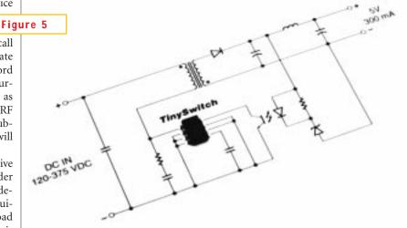
Using the Tinyswitch from Power Integrations as the core, you can build a wall adapter/recharger that is smaller, lighter, and far more efficient than traditional designs, especially in the common but highly wasteful no- or low-load modes.
