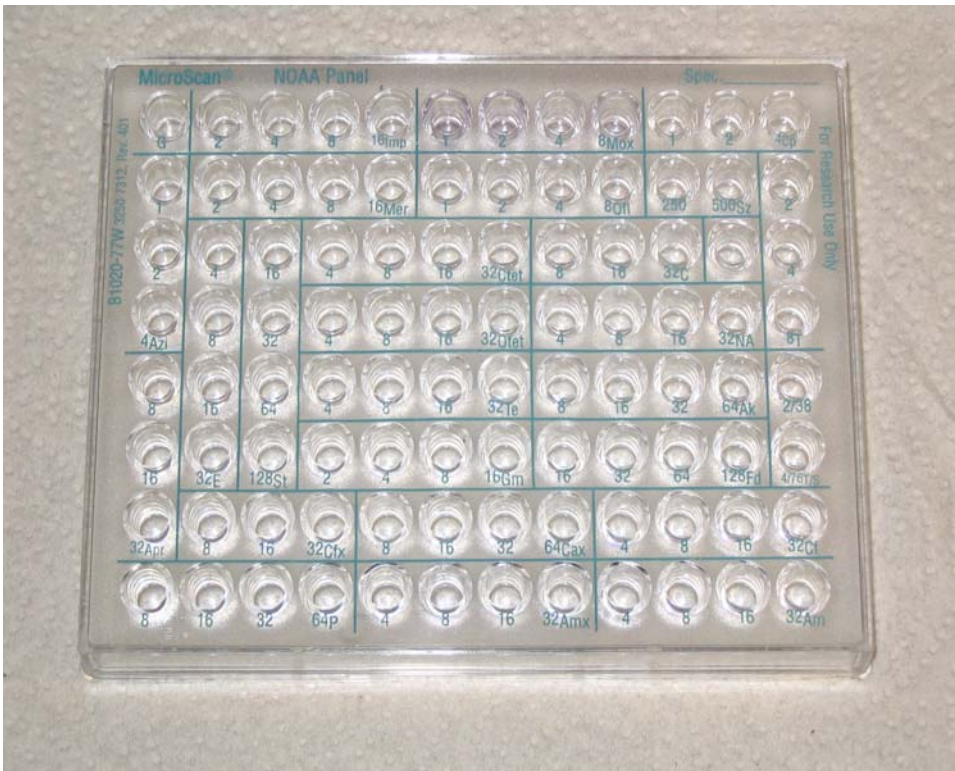
Figure 5. The 96-well suspension plate, containing a preset panel of desiccated antibiotics, designed by Dade Behring specifically for the National Oceanic and Atmospheric Administration (NOAA) (Dade Behring, California).
