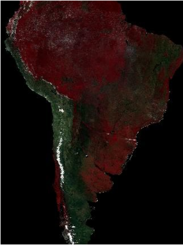
Figure 1. 16-day Composite SeaWiFS GAC image of South America (green, red, and NIR reflectances; bands 4, 5, and 8, respectively).
