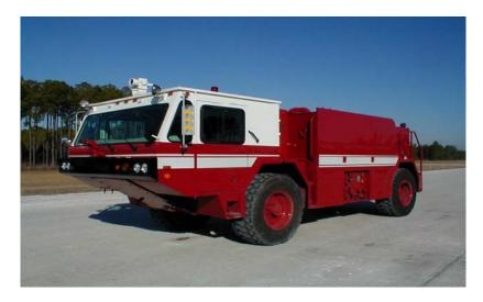
FIGURE 2. UNITED STATES AIR FORCE P-19 WITH ROOF-MOUNTED TURRET
