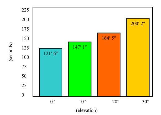
FIGURE 19c. THE HIGH-PERFORMANCE, MULTIPOSITION, BUMPER-MOUNTED TURRET WATER STREAM THROW RANGE TESTS, SET TO FULL-UP POSITION AT VARIOUS DEGREES OF ELEVATION
