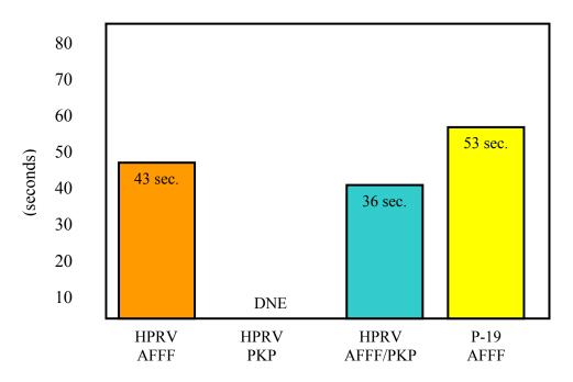
FIGURE 14. AVERAGE RESULTS OF THE TAIL-MOUNTED, HIGH ENGINE NACELLE FIRE TESTS
