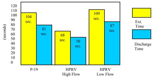
FIGURE 18. AVERAGE RESULTS OF THE LARGE-SCALE POOL FIRE TESTS
