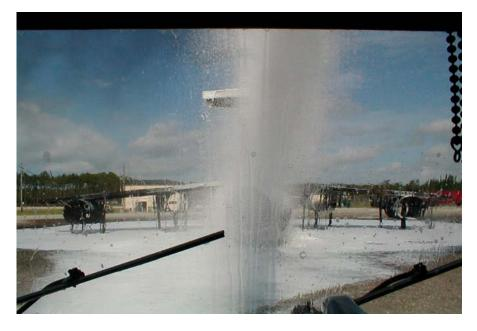
FIGURE 17. THE P-19 ROOF-MOUNTED TURRET USING AFFF
