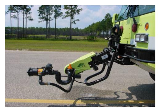
FIGURE 3. THE HPRV WITH 500-gpm HIGH-PERFORMANCE, MULTIPOSITION, BUMPER-MOUNTED TURRET
