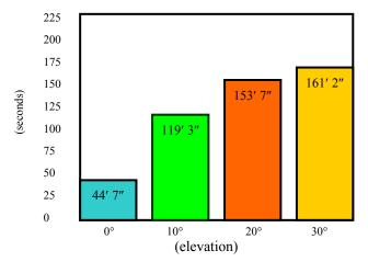
FIGURE 19a. THE HIGH-PERFORMANCE, MULTIPOSITION, BUMPER-MOUNTED TURRET WATER STREAM THROW RANGE TESTS, SET TO DIF POSITION AT VARIOUS DEGREES OF ELEVATION
