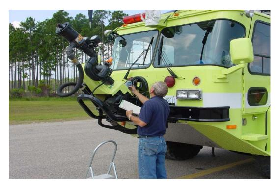
FIGURE 9. THE HIGH-PERFORMANCE, MULTIPOSITION, BUMPER-MOUNTED TURRET FULL-UP POSITION WITH THE TURRET AT 30°
