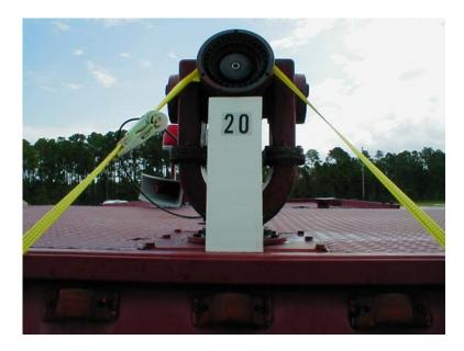
FIGURE 11. THE P-19 ROOF-MOUNTED TURRET JIG SET AT 20°
