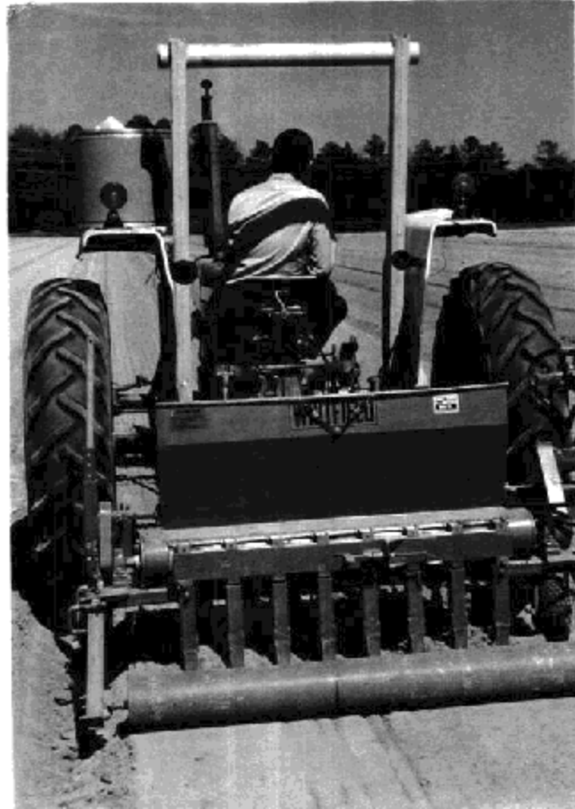
Figure 3. Applicator for mycorrhizal fungus inoculations in bare-root nurseries.
