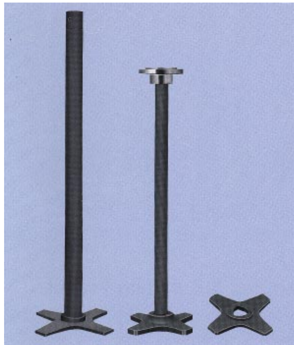
Fig. 7.6. Silicon nitride degassing pipe and rotor used to stir molten aluminum and bubble gases for removal of hydrogen. Source: Kyocera Corporation, Kyoto, Japan.
