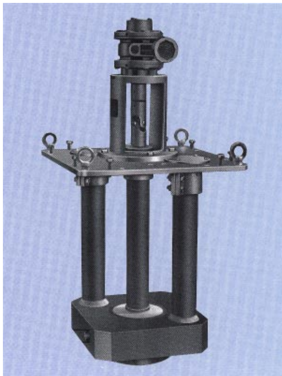
Fig. 7.7. Pump for transfer of molten aluminum, constructed with silicon nitride shaft, impeller, body column, liner ring, and casing liner. Source: Kyocera Corporation, Kyoto, Japan.
