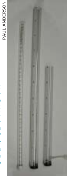
Three different styles of transparency tube—the Ohio Sediment Stick (left), GLOBE tube, and Minnesota Pollution Control Agency tube—were compared in a study by Anderson and Davic at Ohio EPA.
