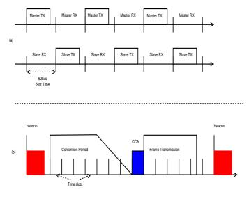
Fig. 1. WPAN structure: (a)Bluetooth (b)Slotted 802.15.4
