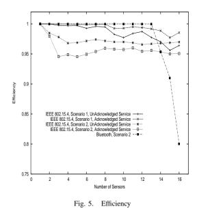
packet on the transmitter side. Even if the drop rate is small (about 1% when 3 or more sensors are used), it is a major disadvantage when using medical applications with strict loss requirements.
