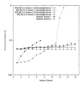
Fig. 3. Delay as a function of number of sensors
