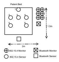
Fig. 6. Heterogeneous Wireless Environment
