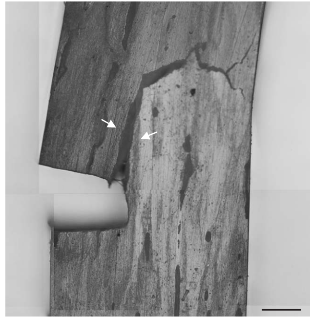
Figure 3. Optical micrograph illustrating \sim 90^\circ crack deflection for an L-C oriented specimen into the longitudinal direction (indicated by white arrows) along a cement line in human cortical bone taken from the humerus.
