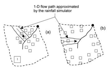
Figure 2. Spatial arrangement of impervious elements on the experimental watersheds for: (a) elements "connected" to the stream channel, and (b) elements "unconnected" to the stream channel.
