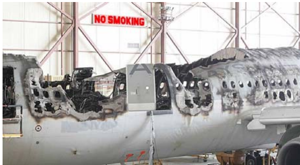
In-flight thermal damaging
