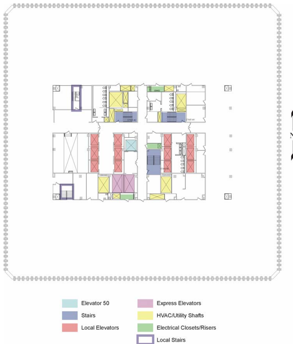
Figure 4–1. Floor layout, 95th floor, WTC 1.
