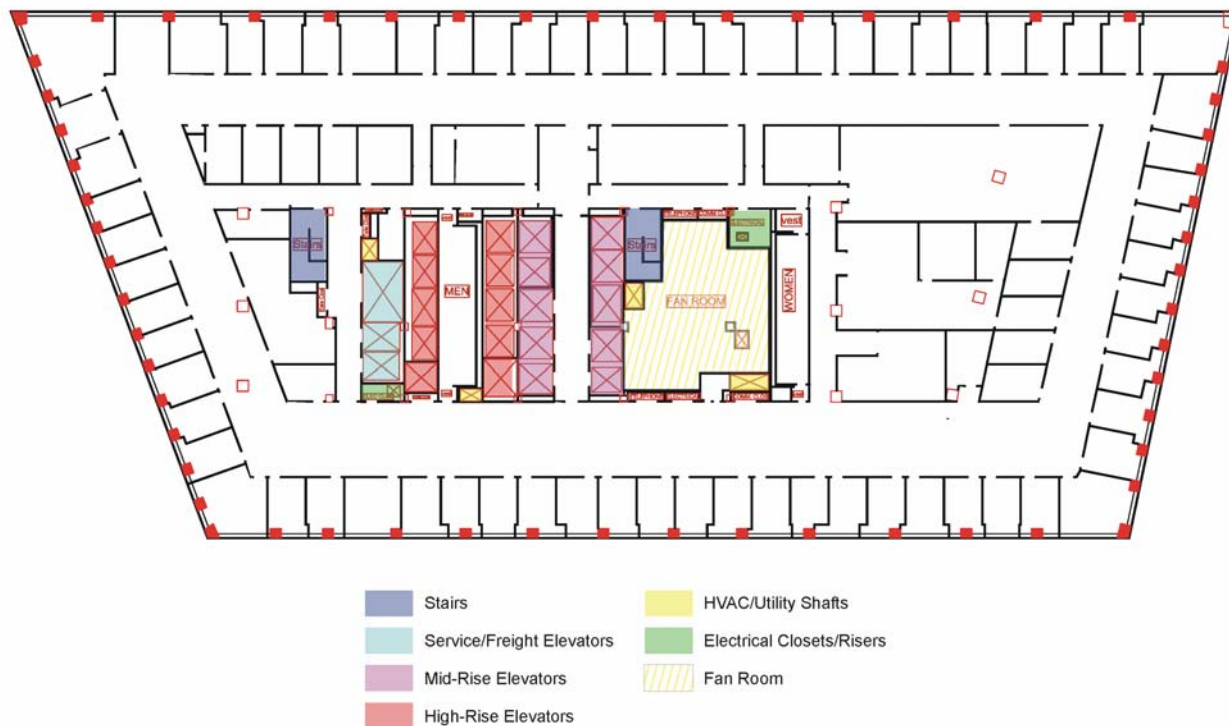
Figure 4–10. Floor layout, 24th floor, WTC 7.
