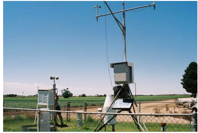
Image of the weather station at NMSU-ASC monitoring daily meteorological conditions including evaporation rate, relative humidity, solar radiation and temperature.
