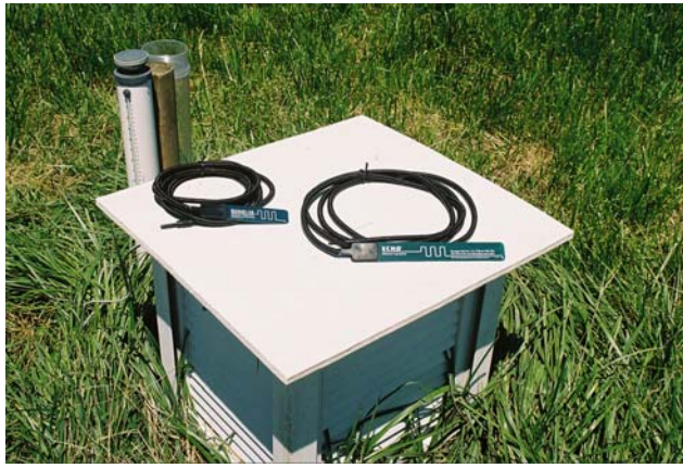
Image of an evapotranspiration gage, two soil moisture probes and a soil moisture data logger field box located at the head of the Bench 3 fescue pasture, NMSU-ASC.
