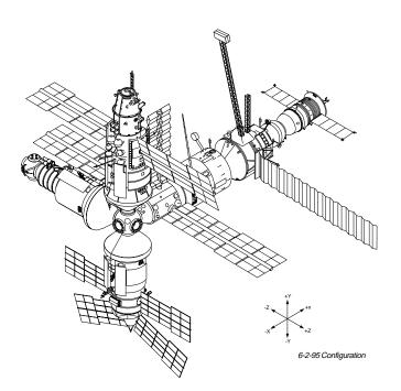
Figure 8. The Mir complex as configured after multiple relocations of Kristall to accommodate Spektr docking and subsequent relocation to the -Y port on June 2, 1995. Spektr is shown at the bottom of the complex in this orientation. July 22 - September 4, 1995
