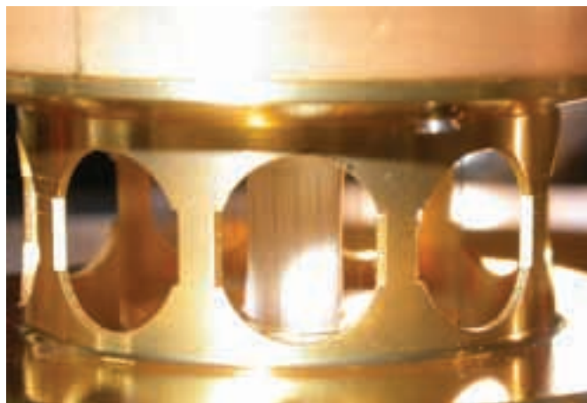
View of a cylindrical wire array and foam target through the oval diagnostic slots of the outer anode can.
