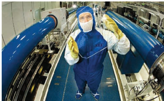
Technologist Benjamin Thurston examines the debris shield that protects the giant Z-Beamlet laser's final focusing lens from flying debris when the Z-accelerator fires.
