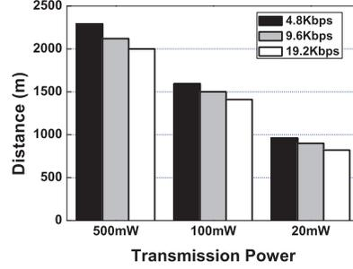
(b) Maximum communication distance at different transmission powers for different rates of EE radio.
