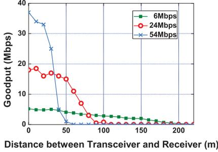
(a) Measured goodput at different distances for different rates of WiFi radio.
