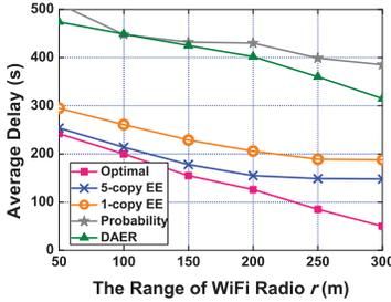
(d) Average delay of 4 routing algorithms when the short range  $r$  varying from 50m to 300m.
