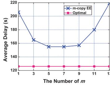
(e) Average delay of m-copy EE routing algorithm when  $m$  varying from 1 to 13.
