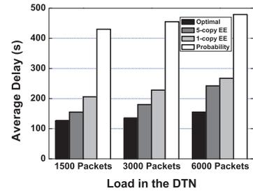
(f) Average delay in different transmission load DTNs. 1500, 3000, 6000 packets are generated in the first 5 minutes in the network.
