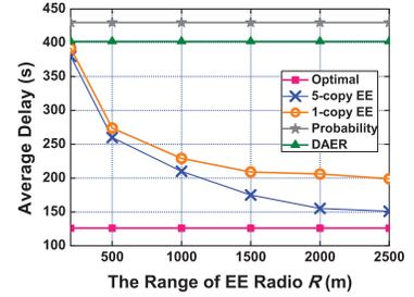
(c) Average delay of 4 routing algorithms when the long range  $R$  varying from 200m to 2500m.
