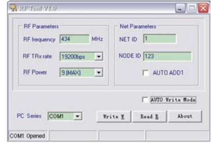
(c) The user interface of the tool we designed to control the parameters of the EE radio.
