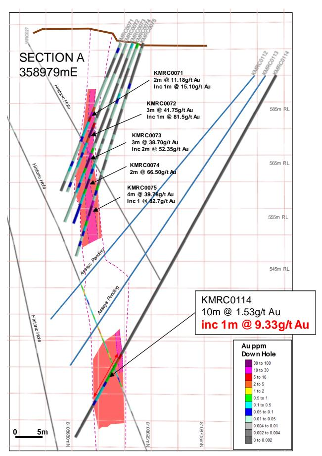
Figure 3 Figure 1 Cross Section- 358979mE, looking west, showing new high grade gold result for KMRC0114. Pink zone >5g/t, red >0.1g/t Au, dashed line broad structure.
