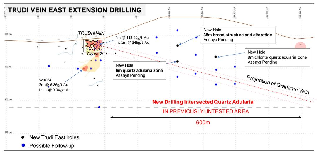
Figure 4: Long Projection, looking north, showing know extents of the Trudi Vein with Trudi high grade area currently being grid drilled (black box – figure 3) and intersection with Grahame Vein plunging to east. Intersections to east previously announced in KRC ASX announcement 12/6/18.
