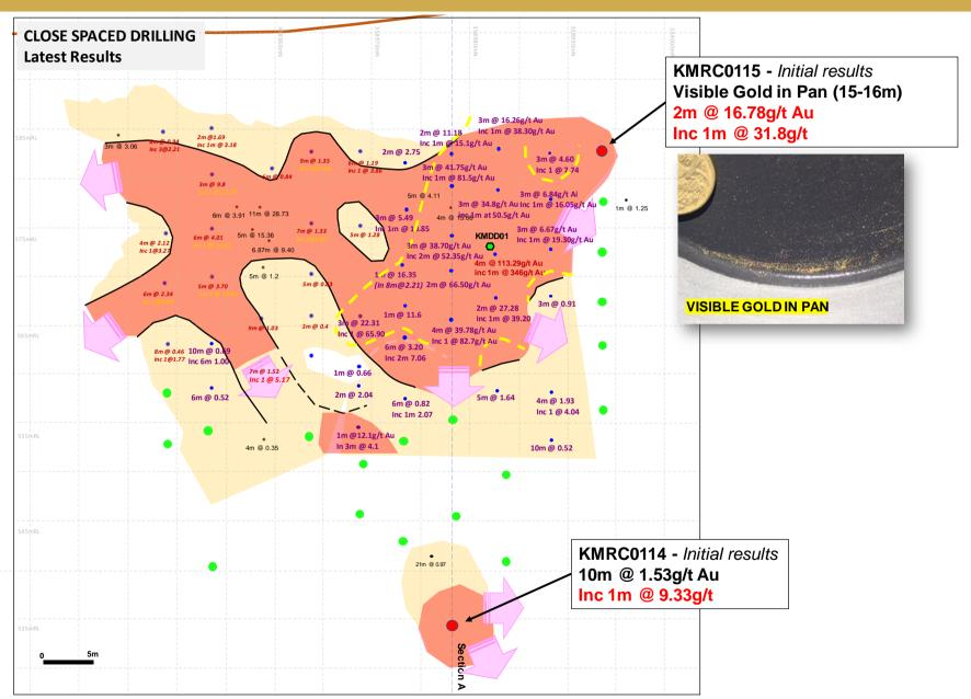
Figure 2: Long Projection, looking north, of Trudi high grade area targeted by close spaced drilling: new very high grade down hole intersects (in text boxes), drilled holes (blue dots), holes with assays pending (green dots), diamond drill hole – green hexagon, > 10 gram metre of gold (red polygon), yellow – 1gram metre.
