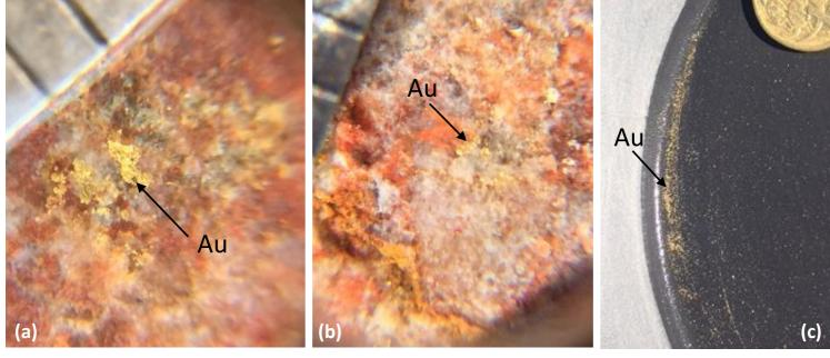
Figure 1 (a) & (b) Photo of visible gold observed in first diamond hole (scale 1mm per bar), (c)- Gold tail in pan from KMRC0115: 15 to 16m (approx. 1kg of RC material panned).
