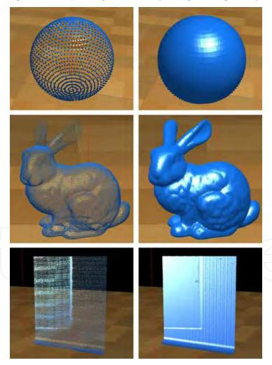
Fig. 10. Splat-rendered objects (Sphere, Stanford Bunny and milled surface containing chatter marks) with low splat size (left) and large splats to make the impression of a closed surface.
