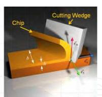
Fig. 3. By casting rays through the chip shape the chip thickness h can be evaluated (left). By the model of the oblique cut (right) the cutting forces can be calculated.
