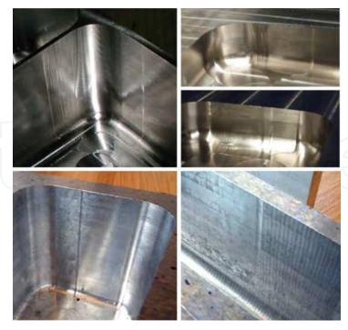
Fig. 1. Typical surface artifacts on milled surfaces. Top left: Marks resulting from changes of feed velocity. Top right: Chatter marks before and in corners. Botton left: Artifact resulting from change of feed direction. Bottom Right: High roughness because of chatter marks.
