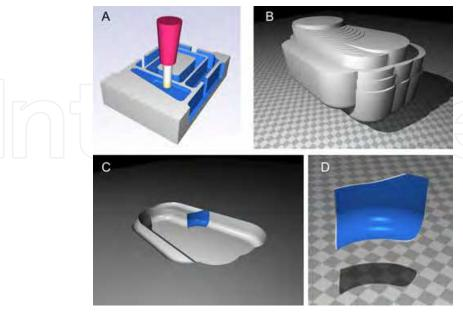
Fig. 2. A local workpiece model (C) at a tool position (A) can be modelled by subtracting the sweep volume (B) of the tool from a stock workpiece. The intersection between this local workpiece and the tool envelope results in the chip shape (D)
