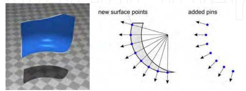
Fig. 6. The exit points of the rays used to compute the chip thicknesses are applied to form a surface model consisting of pins.
