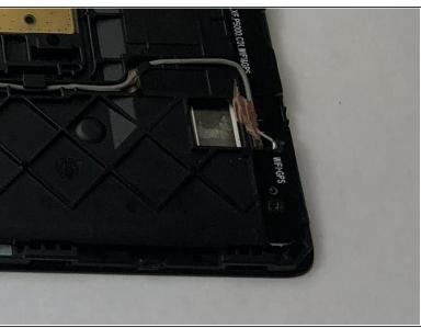
Locate the copper foil holding down the WiFi module near where the grey wire connects. Use tweezers to carefully lift up and separate the copper foil.
