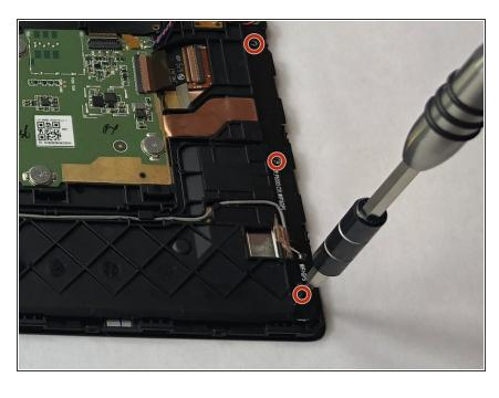
Remove the three 2mm screws holding the wifi module to the device using a PH00 screwdriver.
