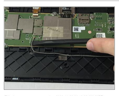
Locate the WiFi module connection on the motherboard by following the grey wire along the bottom. Use a spudger to gently pry it off.
